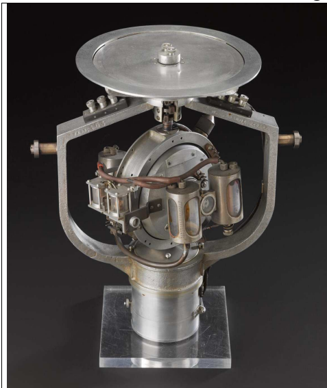
"Original Gyro compass (gyrocompass)" by S G Brown Limited is licensed under CC BY-NC-SA 4.0 .
